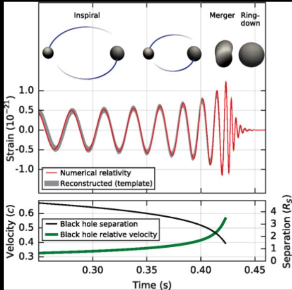
→ source masses, spins, distance, test gravity...
